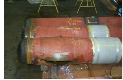
Pipe Body Failure @ 4,260 psi
